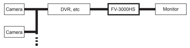
When the image data from a camera is image-optimized and then outputted to a video recorder:
