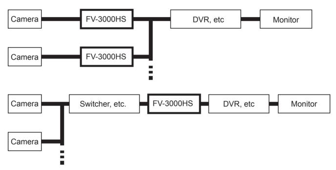
\* Since the I/O signal of FV-3000HS is HD-SDI (BNC), a converter and the like is necessary in case of other signal format.
